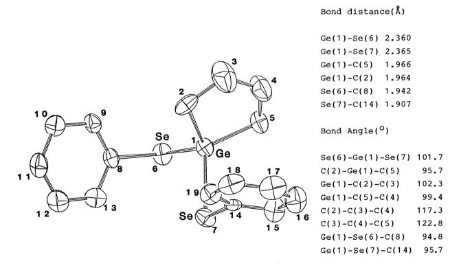
Fig. 1. A perspective view of 1,1-diphenylseleno-1-germacyclopentane (1f) (Hydrogen atoms are omitted), drawn by ORTEP program(see Ref.8). Atoms are shown by 30% probability ellipsoids.
